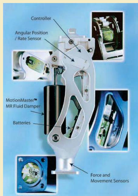
This High Intelligence Prosthesis for the knee uses an MR fluid damper to provide motion that closely duplicates the natural movement of the knee joint.
