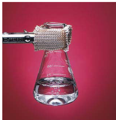
Boiling chip releasing air bubbles acts as a nucleating agent for the bubbles that form when water boils.
